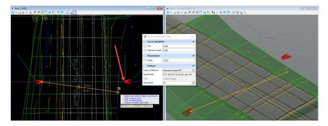
It will model the pipe in the 2D and 3d model at the same time.
