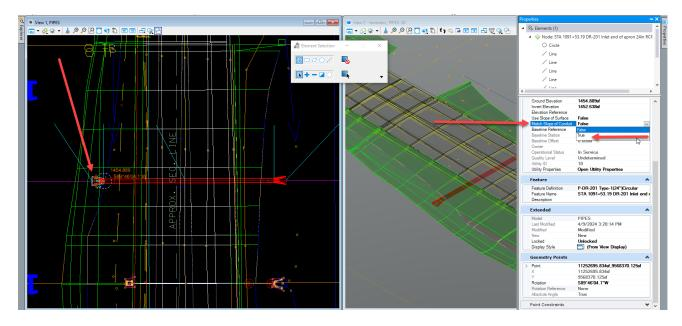
Once the pipe is modeled correctly, delete the smart line created to model the pipe.
