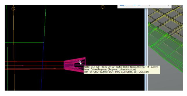
Also, when changes to any of the pipes are required, access the pipe information thru the Explorer tool. It is more efficient to find pipes in large corridor projects by selecting the item in Explorer then right clicking and selecting Fit To View. This will zoom the view to that item.
