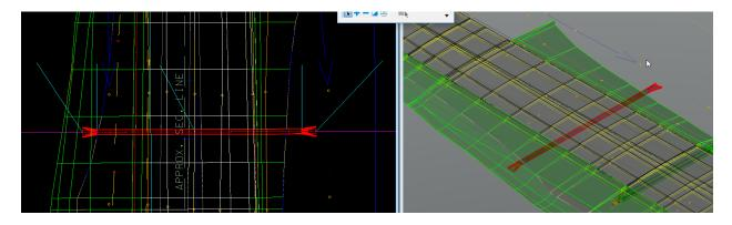
The last step in modeling the pipe is to set the aprons to Match Slope of Conduit. To do this, select the 2D apron node in the 2D model and open the Properties window. Then set the Match Slope of Conduit
